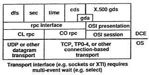
Connection-based transports assume a reliable, sequenced byte stream; message frames are OK
