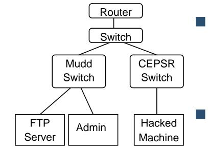
The testing machine was on the same switch as the real server
