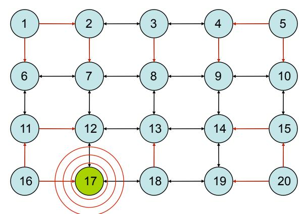
In this case the packet is a TC message but this can be any packet which is to be flooded.
