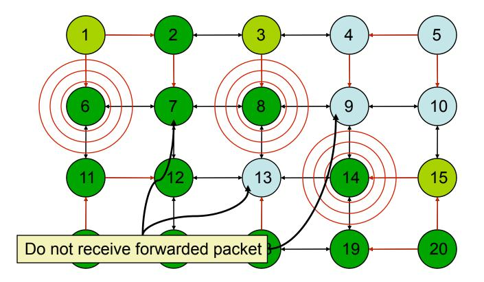
Nodes 15 and 19 receive TC message from 14. Node 3 receives the TC message from 8. Nodes 1 and 11 receive TC message from 6. Nodes 7, 9, and 13 do not receive any TC messages at this time.
