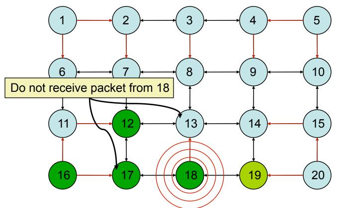
Only node 19 hears TC from 18. Node 13 and 17 do not and should. Node 12 is also forwarding at about this time causing packet collision.
