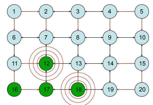
Nodes 12, and 18 resend TC message. Notice that 16 does not because the TC message did not arrive on an arrowed path; this is correct.
