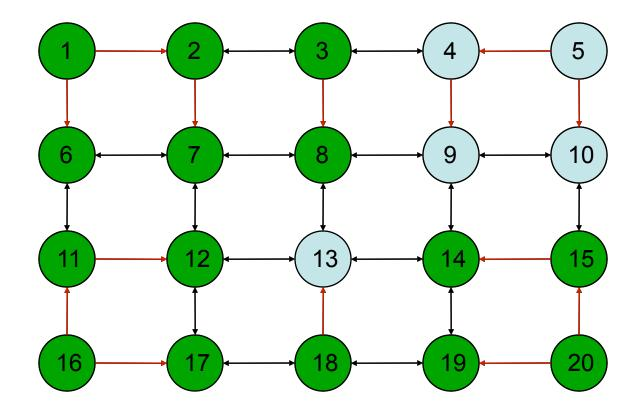
Flooding stops as nodes 1, 3 and 15 are not part of the forwarding path. Nodes 4, 5, 9, 10 and 13 do not receive the flooded packet.
