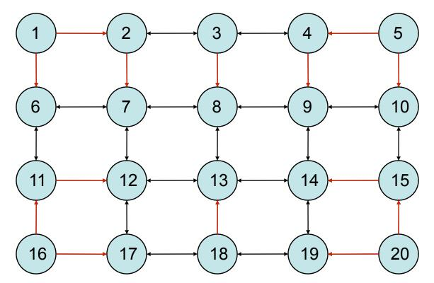
Arrows indicate multipoint relays. A topology control message (TC) sent along an arrow path will be forwarded if that TC was the first received. Red arrows are just highlighting the directional flooding. The forwarding path (MPR nodes) is correct for this network.
