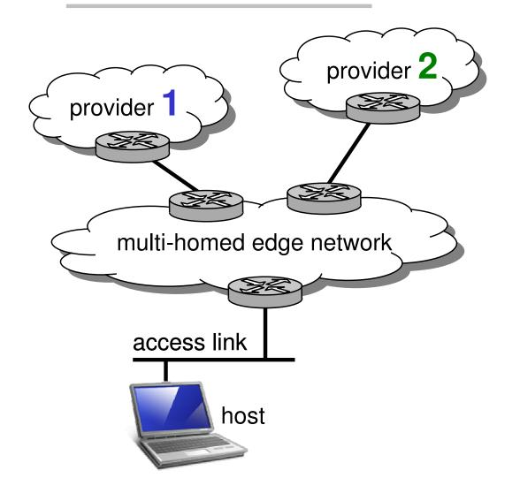
Edge network connects to multiple providers (increased bandwidth, provider services, fault-tolerance) Provider goals
