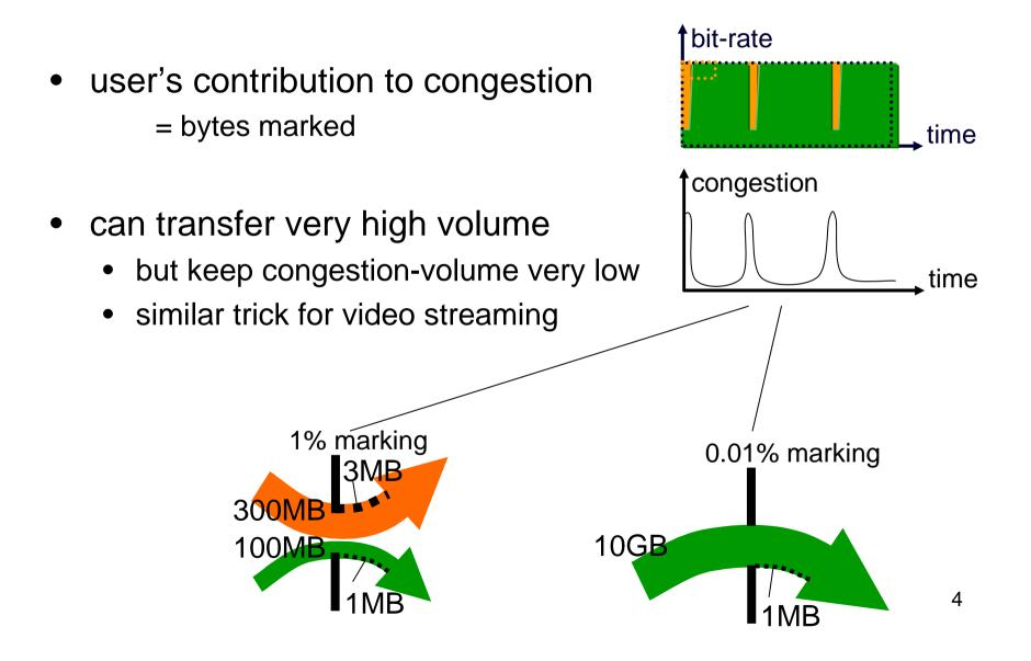
re-inserted feedback (re-feedback) = re-ECN sender exposes congestion to network
