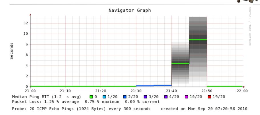
8 second latency over a path of less than 10ms! Much worse than my broadband only test scp of files from my house to expo.x.org, while running speedtest.net Recent commercial home router, 50/10 Comcast service, 9/10/2010
