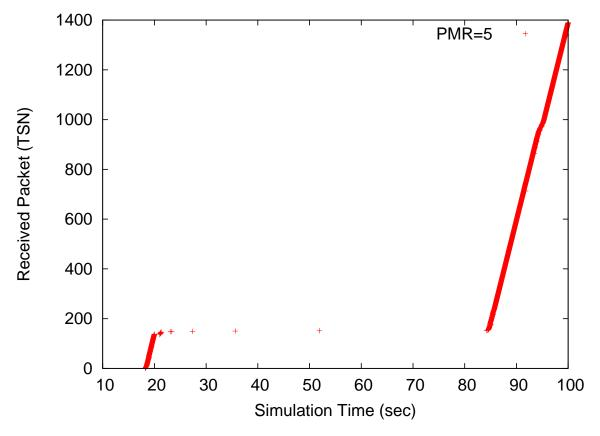
A is sending data to B and B has two address B1, B2 (B1 is primary) when primary becomes unavailable at 20 sec, it takes 60 secs to restart data transmission. (Path.Max.Retrans = 5)
