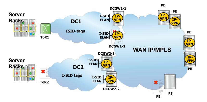
**PBB I-SID tag termination into IP VPN VRFs:** from IP over VLAN to IP over I-SID interfaces
