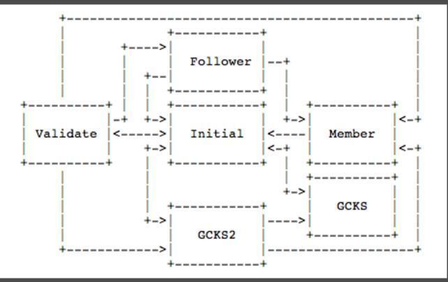
Router starts in Initial state and a router moves through the state machine to either member or GCKS depending on its priority.
