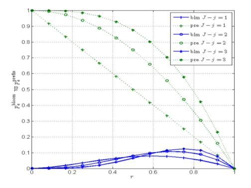
Bloom filter aggregation greatly outperforms the • conventional prefix-based aggregation
