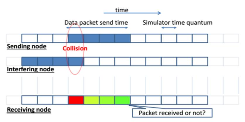
Signal over [noise + interference] averages over packet receiving time => Packet loss probability
