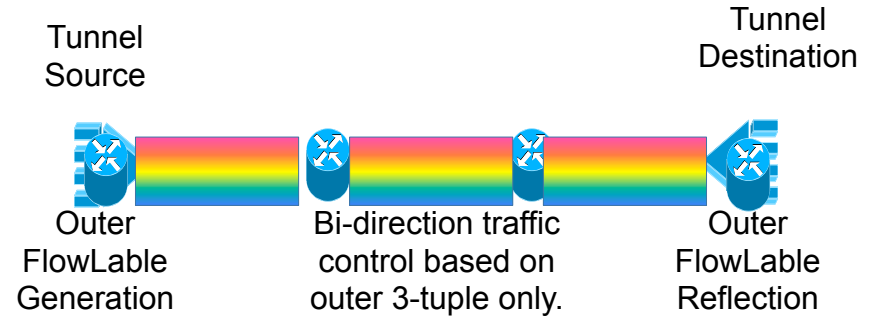
Fig.2 Flow Label Reflection on Tunnel Ends
