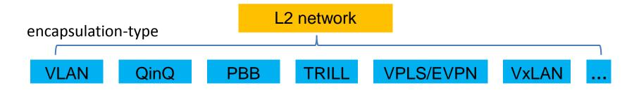
Different layer-2 encapsulations may be used to build one L2
