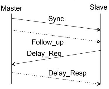
Residence times are accumulated in the associated follow-up messages (or Delay\_Resp message associated with the Delay\_Req message)
