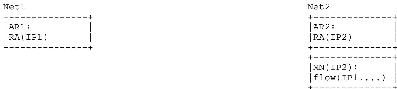
Figure 2. Anchoring function not in network of attachment. MN attached to AR2 in Net2 has a flow(IP1,...) using IP1, which belongs to Net1.
