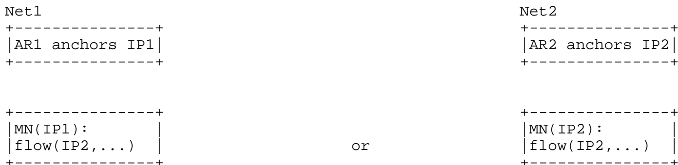
Figure 1. IP prefix/address anchored in network of attachment. MN is attached to AR1 in Net1 where it has initiated a flow using IP1 or has moved to AR2 in Net2 where it initiates a new flow using IP2.
