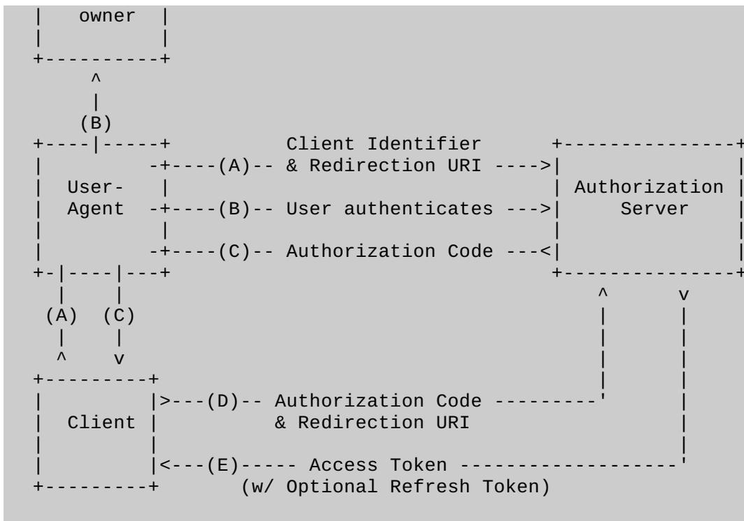
Note: The lines illustrating steps A, B, and C are broken into two parts as they pass through the user-agent.
