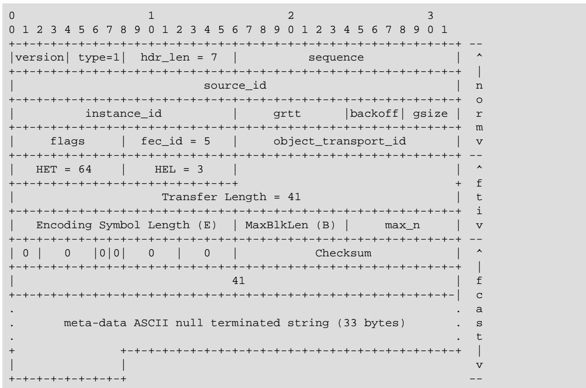
Figure 6: NORM\_INFO containing an EXT\_FTI header extension and an FCAST Compound Object Header
