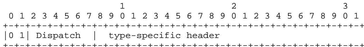
Dispatch                                  6-bit selector. Identifies the type of header immediately following the Dispatch Header.
