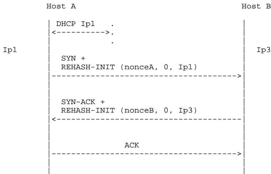
The following diagram shows REHASH-INIT exchange performed by Host B after connection establishment. Should DATA or ACK packets need retransmission, REHASH-INIT options should be sent together with
