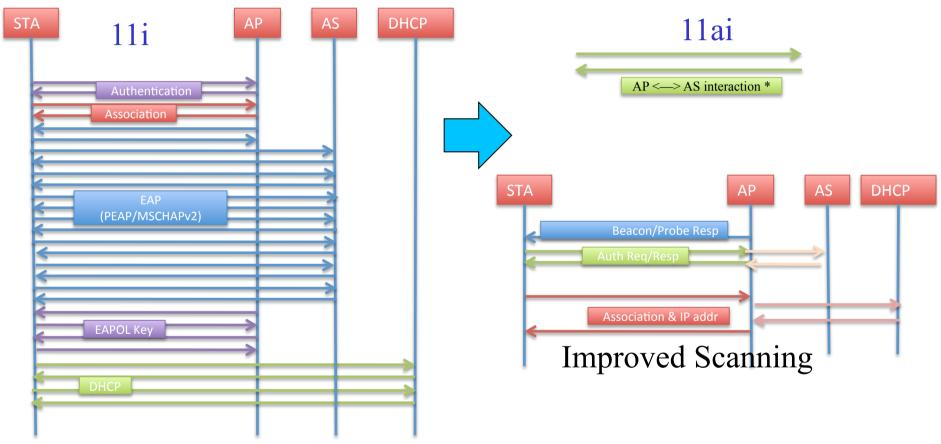
\*Two authentication options are defined. Public key authentication and shared key authentication using ERP. When ERP is used an optional AP <---> AS exchange is required during the FILS exchange.
