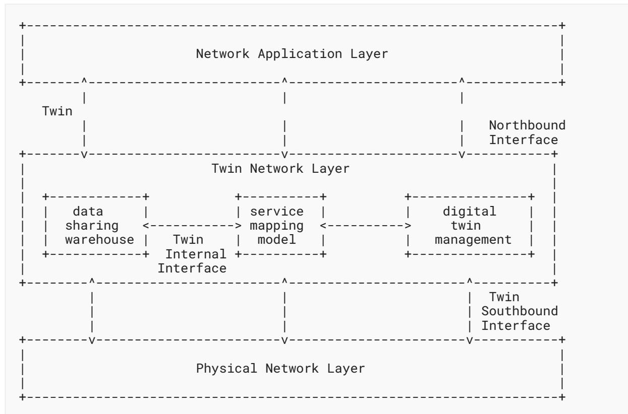
Figure 1: Schematic Representation of DTN Interface
