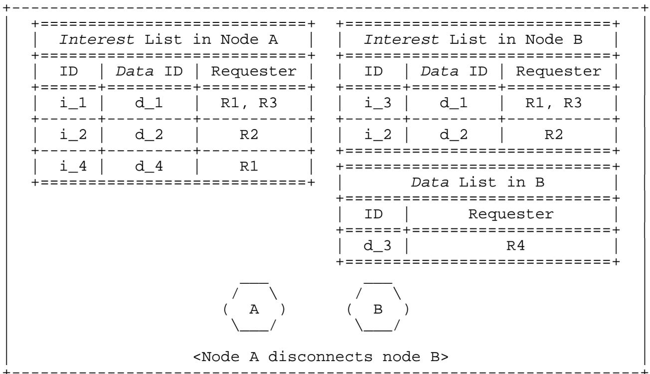
Fig 2. Interest Forwarding Procedure (at time t+dt)
