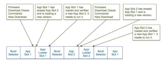
To further reduce this risk, this leads us to prefer the "three loader" approach. This approach extends the "two loader" approach by adding a fallback Loader/Selector that provides a separated means to load Applications/Loaders; in this way, we always have two pieces of software able to perform a load, one of which may recover from more subtle application defects.
