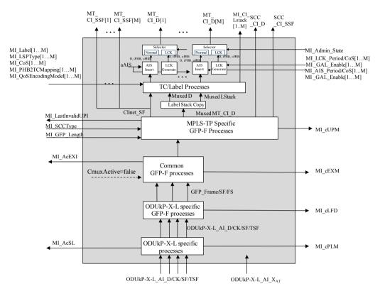
$Figure~11\text{-}27/G.8121/Y.1381 - ODUkP\text{-}X\text{-}L/MT\_A\_Sk~process~diagram$
