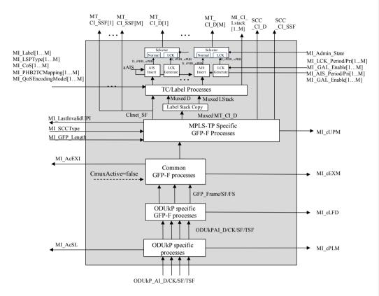
Figure 11-21/G.8121/Y.1381 - ODUkP/MT\_A\_Sk process diagram
