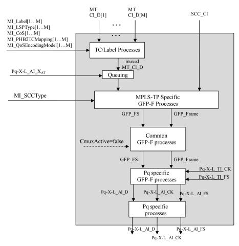
Figure 11-34/G.8121/Y.1381 – Pq-X-L/MT\_A\_So process diagram
