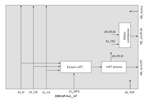
Figure 11-28/G.8121/Y.1341 - ODUkP-X-L specific sink processes
