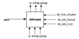
**Figure 8-13/G.8121/Y.1381 – AIS Insert process**
