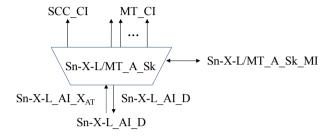
Figure 11-7/G.8121/Y.1381 - Sn-X-L/MT\_A\_Sk symbol
