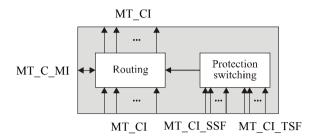
Figure 9-2/G.8121/Y.1381 - MT C process diagram
