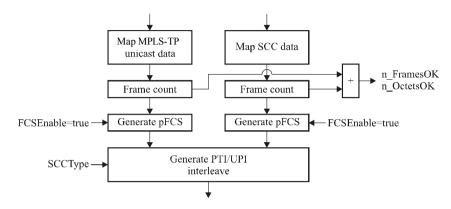
Figure 8-7/G.8121/Y.1381 - MPLS-TP-specific GFP-F source process
