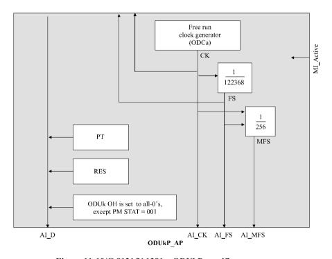
Figure 11-19/G.8121/Y.1381 – ODUkP specific source processes
