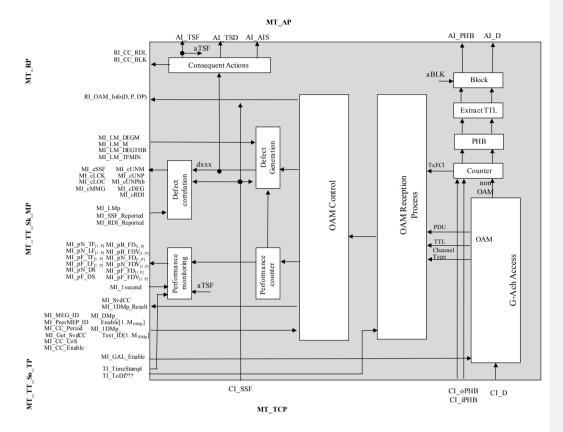
Figure 9-7/G.8121/Y.1381 - MT\_TT\_Sk process diagram
