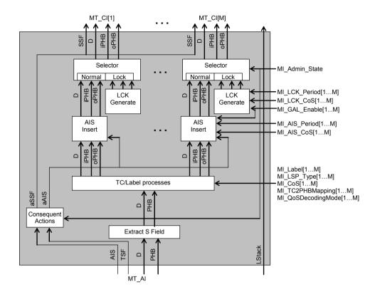
Figure 9-11/G.8121/Y.1381 - MT/MT\_A\_Sk process diagram
