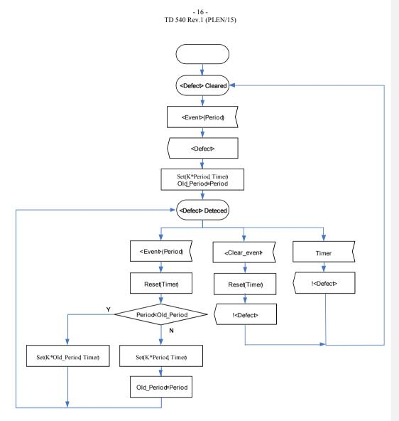
Figure 6-2/G.8021/Y.1341 – Defect detection and clearance process for dMMG, dUNM, dUNP, dUNPr, dAIS, dLCK and dCSF
