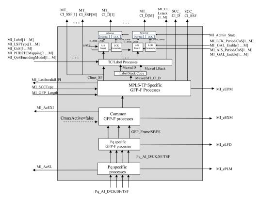
Figure 11-32/G.8121/Y.1381 - Pq/MT\_A\_Sk process diagram
