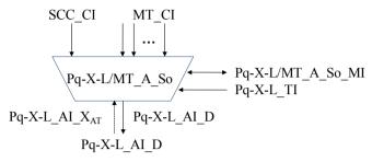
Figure 11-33/G.8121/Y.1381 - Pq-X-L/MT\_A\_So symbol
