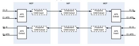
Figure 8-16/ – Overview of the processes involved with APS function
