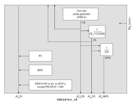
Figure 11-25/G.8121/Y.1381 - ODUkP-X-L specific source processes
