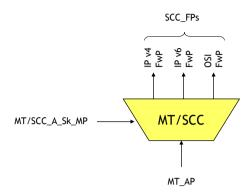
Figure 10-8/G.8121/Y.1382 - MT/SCC\_A\_Sk function
