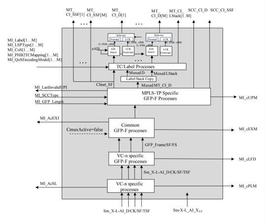
Figure 11-16/G.8121/Y.1381 – Sm-X-L/MT\_A\_Sk process diagram
