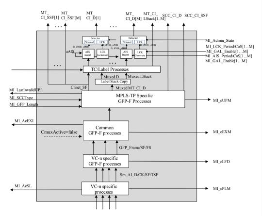
$Figure~11\text{-}12/G.8121/Y.1381 - Sm/MT\_A\_Sk~process~diagram$
