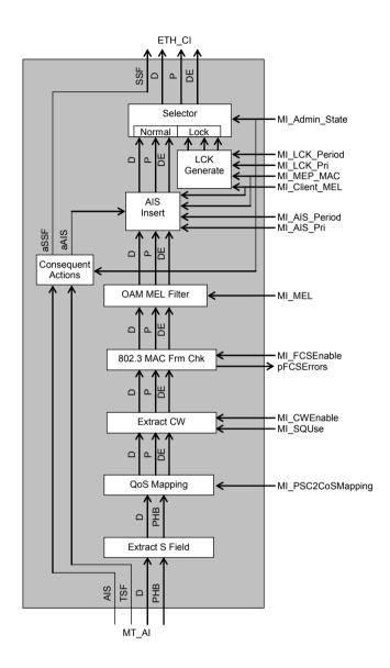
Figure 10-4/G.8121/Y.1381 – MT/ETH\_A\_Sk process diagram
