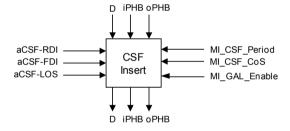
Figure 8-22/G.8121/Y.1381 - CSF Insert process
