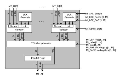
Figure 9-9/G.8121/Y.1381 – MT/MT\_A\_So process diagram
