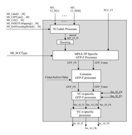
Figure 11-6/G.8121/Y.1381 – Sn-X-L/MT\_A\_So process diagram
