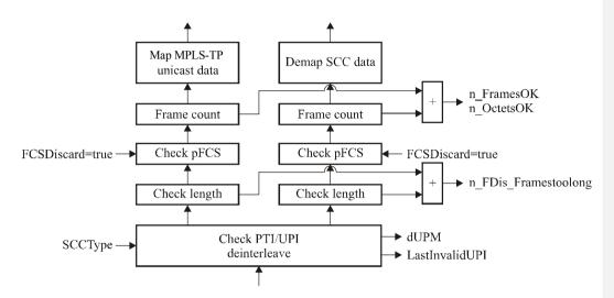
Figure8-8/G.8121/Y.1381 - MPLS-TP-specific GFP-F sink process
