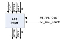
Figure 8-17/G.8121/Y.1381 - APS Insert process
