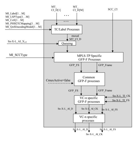
Figure 11-2/G.8121/Y.1381 - Sn/MT\_A\_So process diagram
