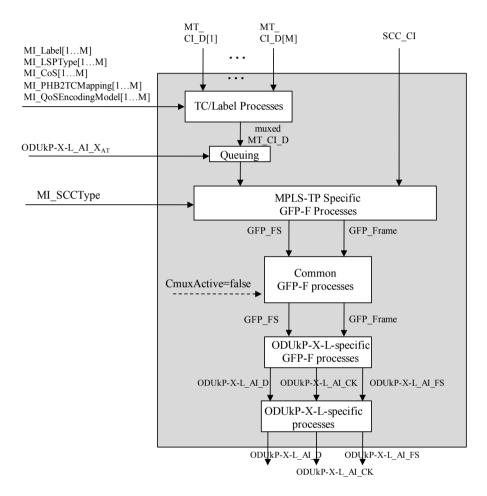
Figure 11-24/G.8121/Y.1381 - ODUkP-X-L/MT\_A\_So process diagram
