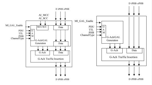
Figure 8-1 - G-ACh Insertion Process
