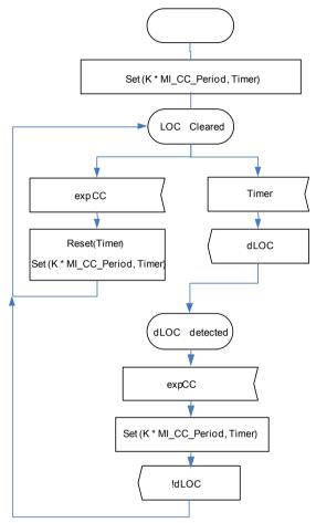
Figure 6-1/G.8121/Y.1381 - dLOC detection and clearance process
