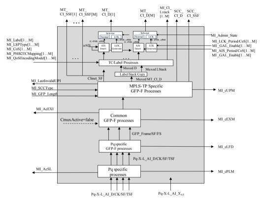
Figure 11-36/G.8121/Y.1381 – Pq-X-L/MT\_A\_Sk process diagram
