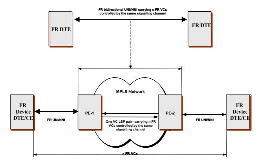
Figure - 9/X.84 illustrates the concept of frame relay many-to-one mapping mode
