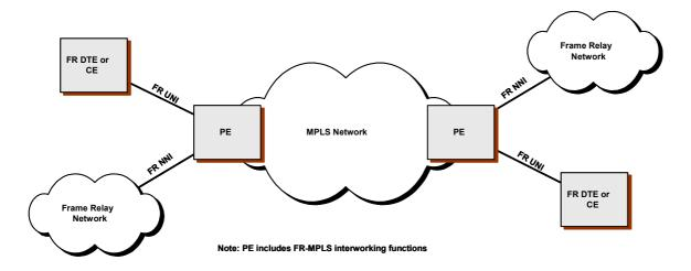
Figure 1/X.84 - Frame Relay over MPLS core network reference model
