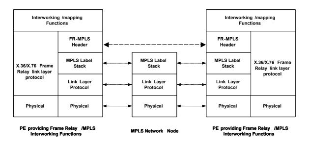
Note: Recommendations X.36 and X.76 supersedes Recommendation Q.922 and contain the same frame relay link layer protocol as defined in Recommendation Q.922 link core service.
