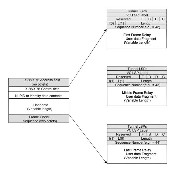
Figure I.1/X.84 – Example of fragmentation for the one to one mapping mode
