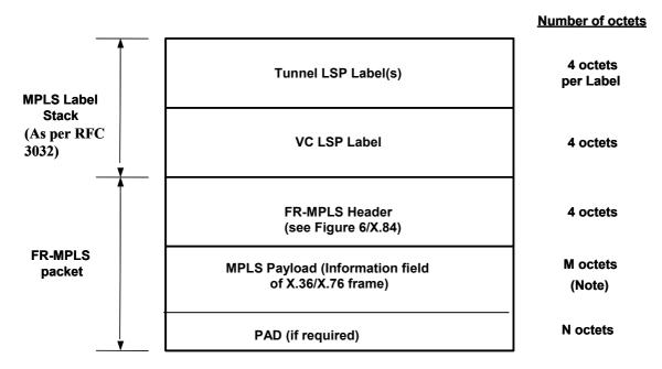
Note: The default number of octets in the payload field (X.36/X.76 frame relay information field only) is defined in Recommendations X.36 and X.76. If it is greater than the MTU, fragmentation may be used.
