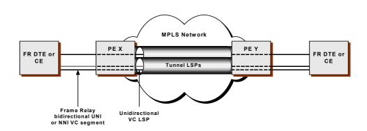
Figure 2/X.84 – Tunnel and VC LSPs
