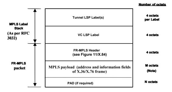
Note: The the payload field includes X.36/X.76 frame relay information field and the address field (including the DLCI and control fields).
