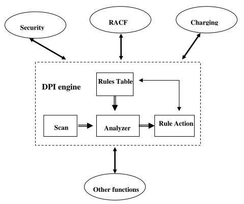
Figure 1. DPI within the packet-based networks and NGN environment
