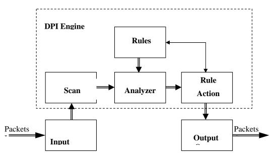
**Figure 2** – The basic DPI function and architecture
