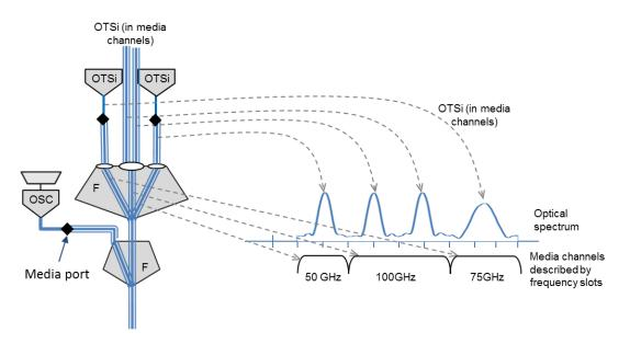
Figure 7-2 – Relationship between signals and media channels
