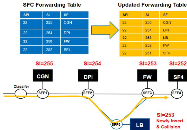
Fig-1 Existed SI assignment mechanism of SFC in mobile scenario
