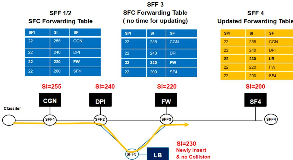
Fig-2 Heterogeneous SI assignment mechanism of SFC in mobile scenario
