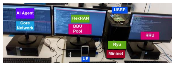
Fig. 8 – Testbed working at LASSE – UFPA lab using a C-RAN architecture.
