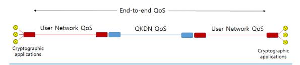
Figure 7. End-to-end QoS domain for cryptographic applications
