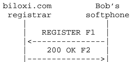
Figure 9: SIP Registration Example
