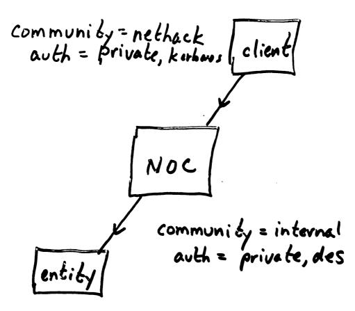
monitored entities are simple complexity and access control centralized at NOC
