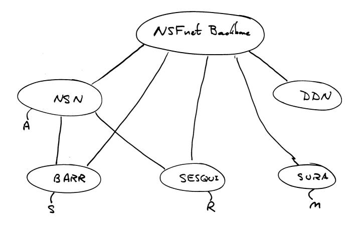
Essentially a DAG Vertices are Autonomous Systems Aves are Inter AS connection Realizing Exclanges Two-place rule: Elip's EDown?
