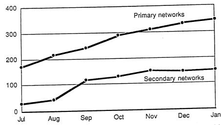
HIGHLIGHTS: The NSFnet is a policy-based system. It will only let authorized traffic pass through the backbone. This chart represents "configured" networks in the NSFnet. At the beginning of July about 180-190 nets were configured, with growth to 360-370 networks allowed by the first of January 89.
