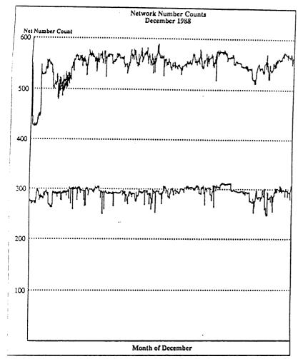
HIGHLIGHTS: Throughout December the total count tends to grow quite significantly. At about the 570 Net Number Count was the time at which deployment of the butterflies was needed. That level was exceeded before the butterflies were deployed but they are now in place and operating.
