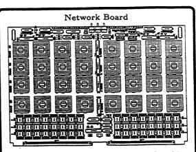
Contains 16 port network. PSE chips packaged in 108 pin PGAs.
