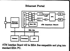
Ethernet Controller transfers packets to/from dual-ported memory on ATM Interface Board.
