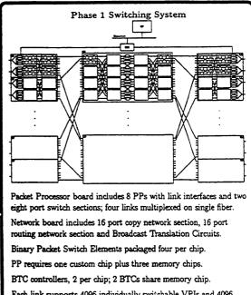
Each link supports 4096 individually switchable VPIs and 4096 VCIs; system supports total of 4096 multicast connections.
