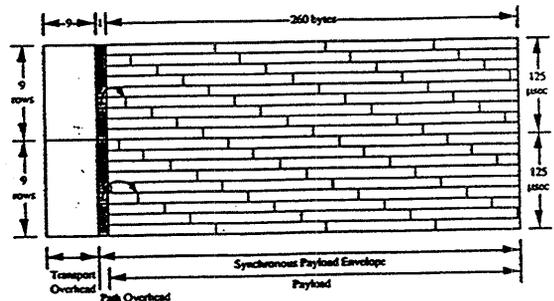
$$\frac{260 \text{ bytes} \times 8 \times 9}{125 \mu\text{sec}} = 149.760 \text{ Mb/s}$$
