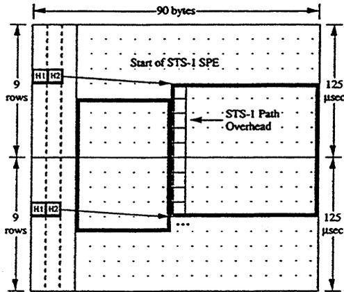
H1 & H2 pointers in Line Overhead used to adjust for "slips" and "stuffs" across plesiochronous boundaries. SPE may begin anywhere within 125 μsec STS-1 frame.
