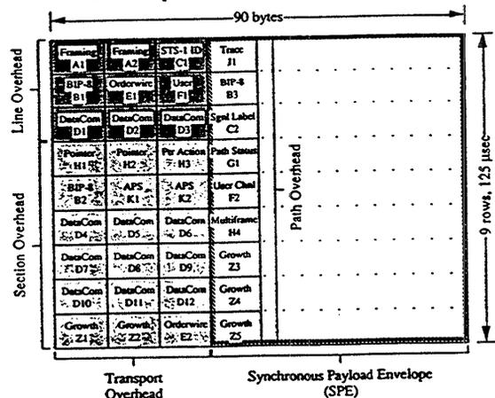
9 rows × 90 bytes × 8 / 125 μsec = 51.840 Mb/s line signaling rate.
