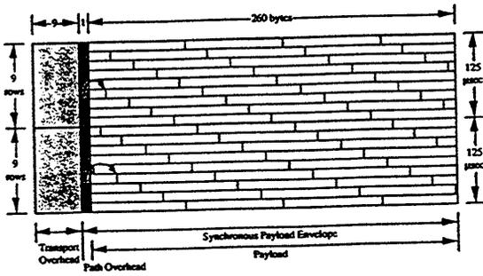
$$\frac{260 \text{ bytes} \times 8 \times 9}{125 \mu\text{sec}} = 149.760 \text{ Mb/s}$$
