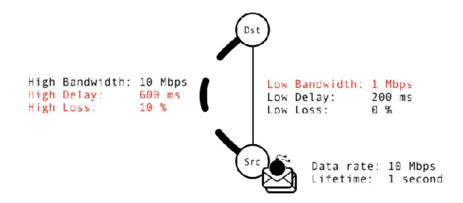
Sending initially the data along the left-hand path and retransmitting lost packets along the right-hand path, we can expect to deliver **100% of the packets** before their deadline.
