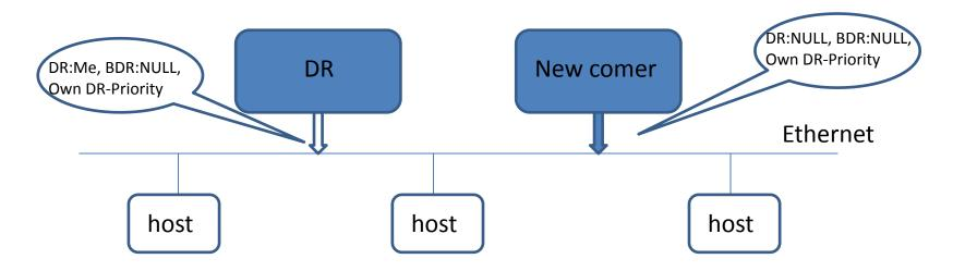
• When a new router which have no DR-improvement capability comes in, the new router sends the hello packet with it's DR-priority at first.
