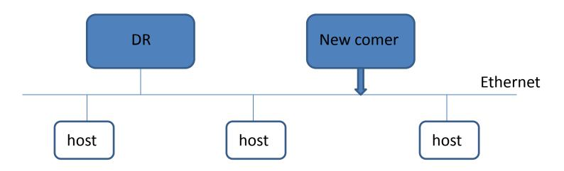
•When a new router which have higher DR-priority comes in, the new router will become the DR and import multicast flow from upstream router.
