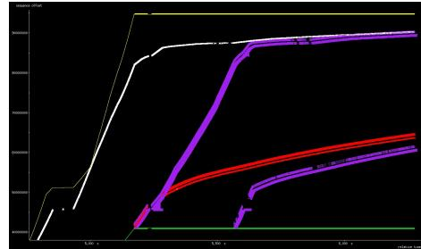
Paced TCP CUBIC on a 10Gbps WAN path with RTT=308ms. Fast recovery at end of initial slow start.
