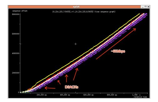
TCP-BBR on 100Mbps w/ rand[15ms,25ms] RTT. TCP is constantly in (false) recoveries (**R** is retransmission, (D)SACK is purple)
