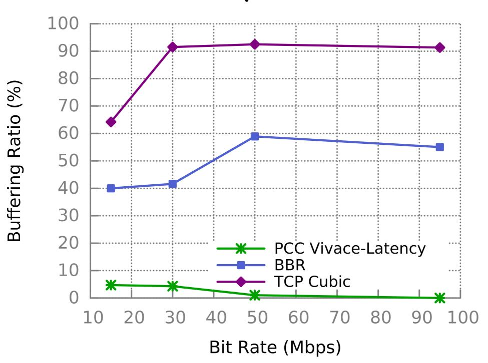
3 competing streaming flows on bottleneck link with 75KB buffer, 100ms RTT, 0.01% random loss, and adequate bandwidth
