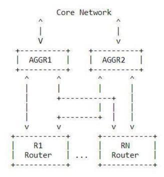
Reverse-Metric mechanism allows AGGR1 to signal R1 to increase its metric towards AGGR1 such that the path via AGGR2 becomes the preferred path.
