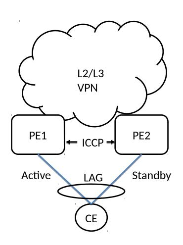
Following picture shows a typical MC-LAG topology using ICCP to drive the active-standby state on peering routers.
