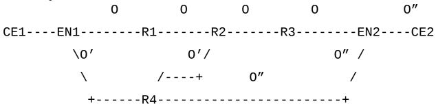
The replication sub-function creates copies of the OAM packet at nodes EN1 and R4.
