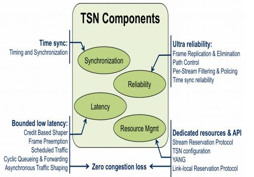
Time Sensitive Networking is an enhancement to IEEE 802 networks enabling the convergence of real-time control with time-critical streaming and and bulk data into a single communication network.
