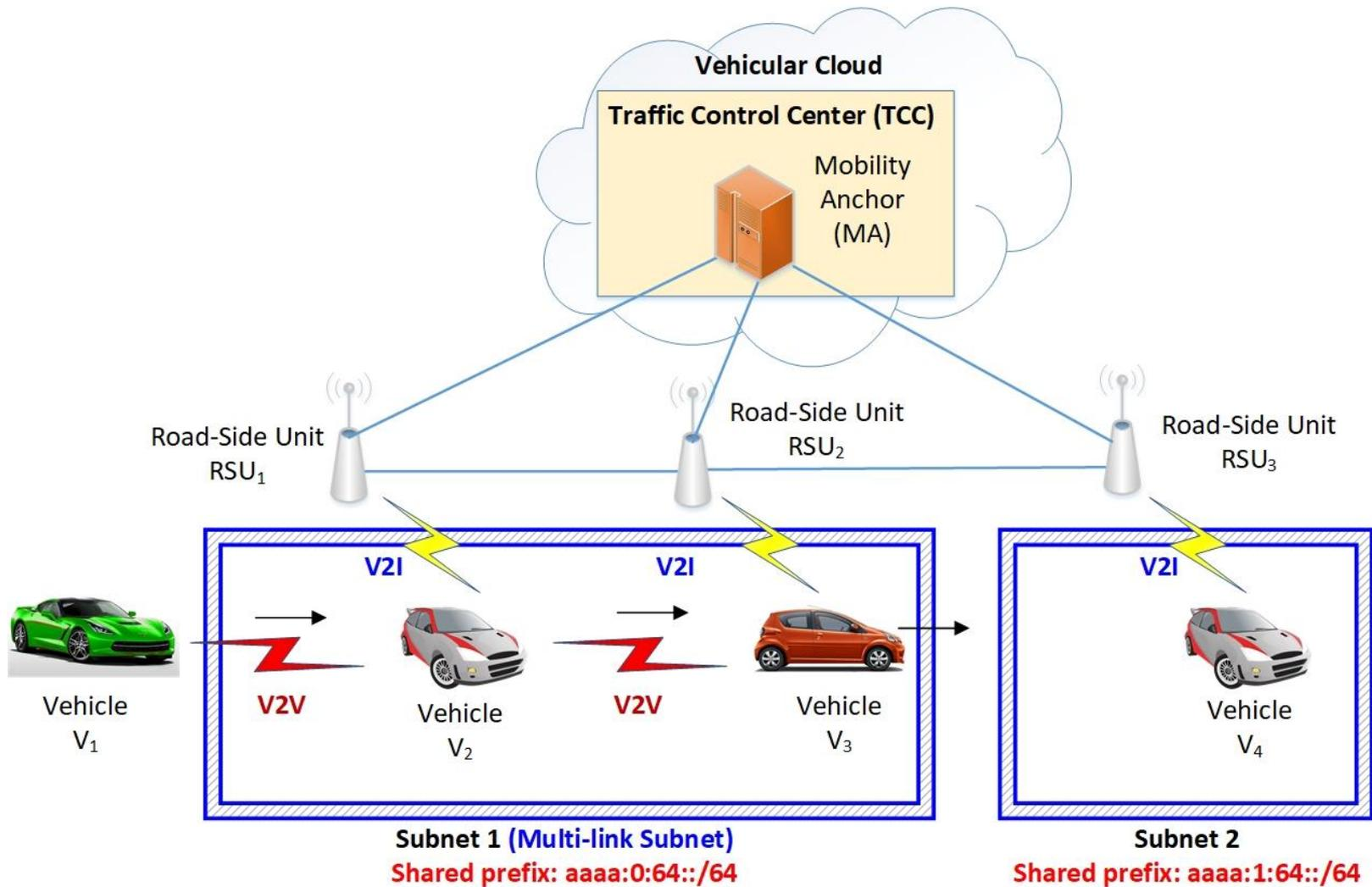
Figure 1: A **Vehicular Network Architecture** for V2I and V2V Networking
