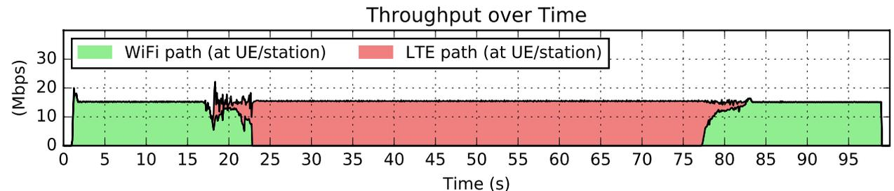
Additionally to the scenario on top, using path aggregation combined with path prioritization on WiFi enables a smooth handover, keeping QoS stable
