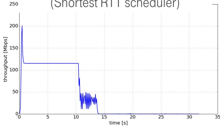
Path usage: a break in cheapest path (immediately visible at sender) at 10s, path back up at 23s
