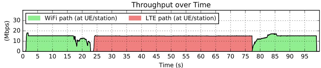
After detecting the physical loss, stream is handed over to cellular without connectivity break
