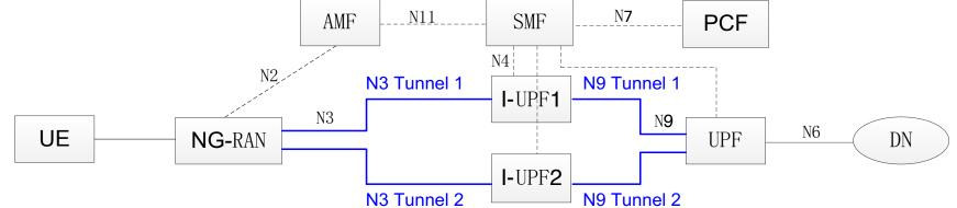
Reference: 3GPP TR 23.725 Figure 6.4.1-2 Two N3 and N9 tunnels between NG-RAN and UPF for redundant transmission
