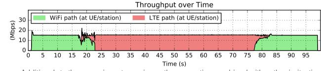
Additionaly to the scenario on top, using path aggregation combined with path prioritzation on WiFi enables a smooth handover, keeping QoS stable
