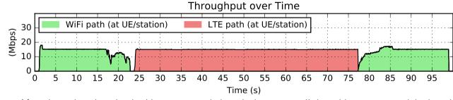
After detecting the physical loss, stream is handed over to cellular without connectivity break.
