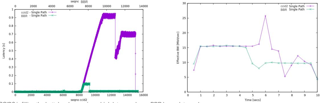
CCID2 is filling the bottelnecks causing a high latency wheres BBR keeps latency low.
