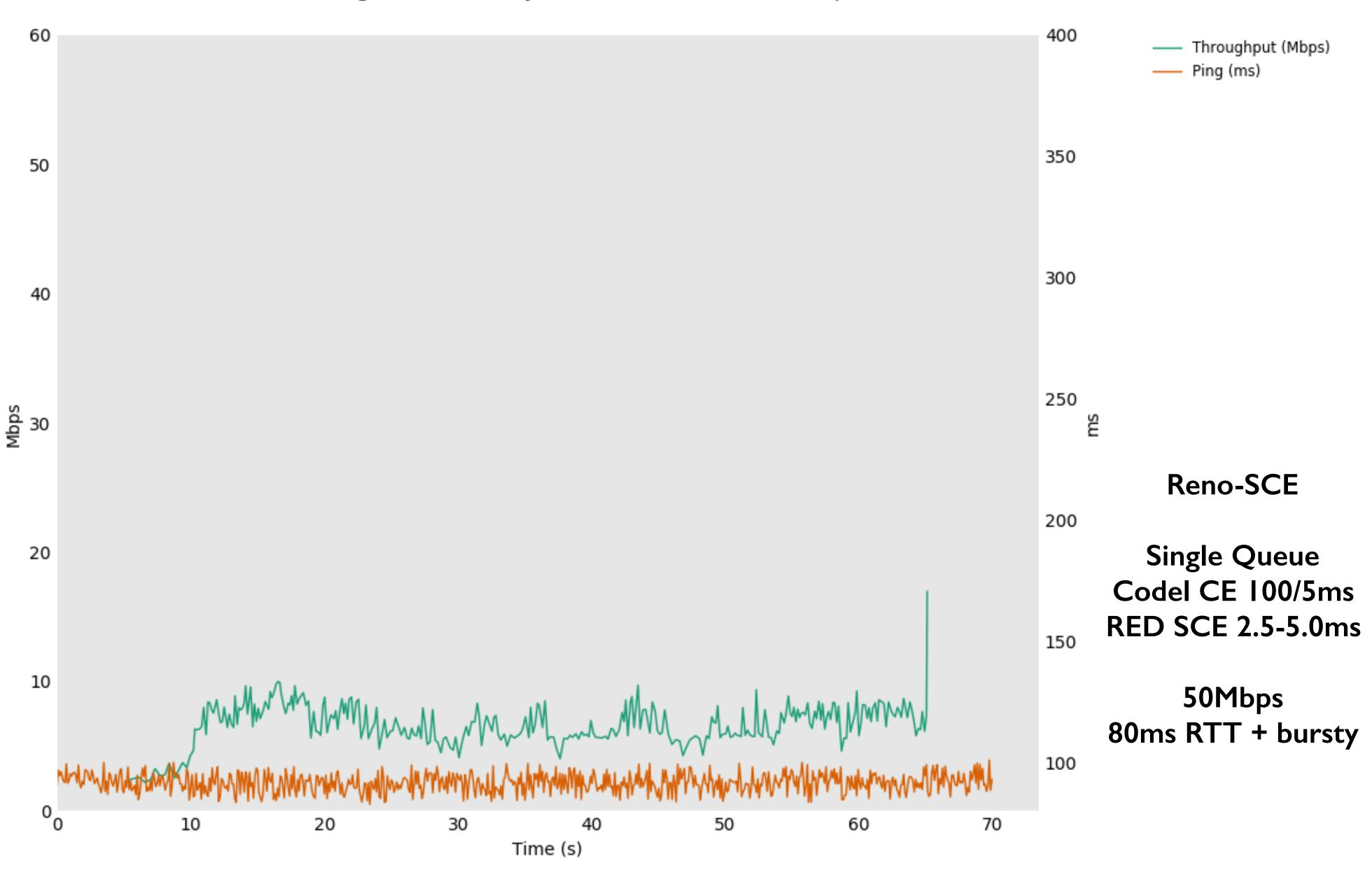
TCP Reno-SCE w/ping through simulated 50Mbps/80ms bursty link (CNQ) Sender (reno-sce) → 80ms delay + slotting → CNQ 50Mbit → Receiver slotting: netem delay 200us slot 800us 10ms packets 32
