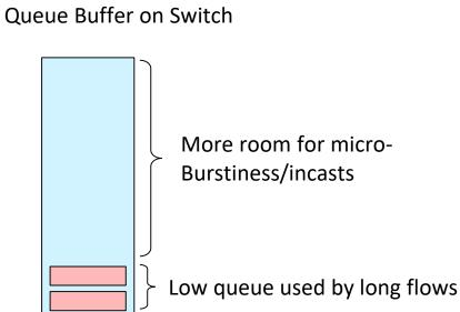
Small queue size reduces queueing delay and packet loss, so LDCP is not specific to RoCEv2, but is open to all transports with a reliable service
