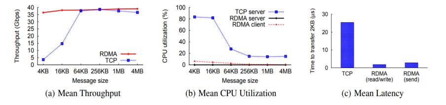
RDMA outperforms TCP in throughput, CPU utilization and latency
